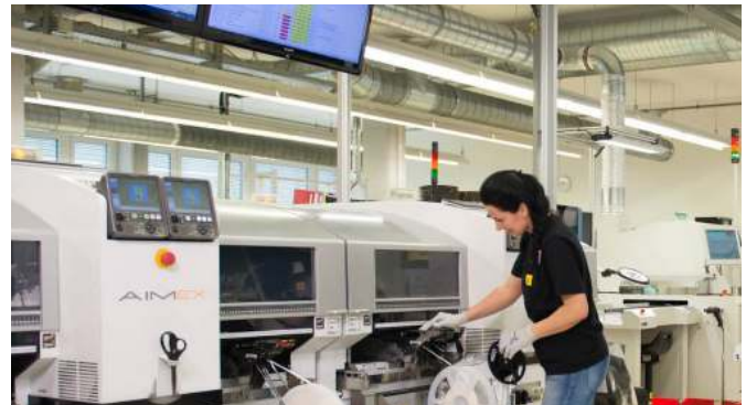
SMT Assembly – Assembly of up to 100 components per single board a lateral precision accuracy < 40 micrometers
